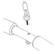
Thread the bolt with the ropes to hang the swing through the holes on the completed ring, and fasten.
