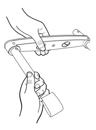
Take the lower half of the ladder and insert the ends with the push buttons inside the hook poles. Push the buttons down to allow the hook poles to slide over the middle poles until the buttons pop out.
