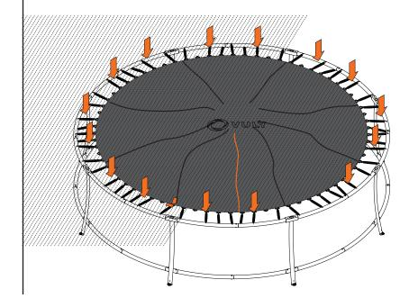
**NOTE:** Attach one Spring either side of the middle Springs using the Spring Tool. Beware of alternating spring position.
