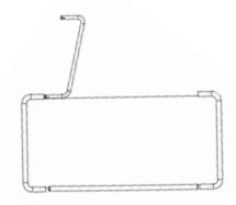
**B.** Slide the straight Frame Tubes through the holes along the side of the Base Material.
