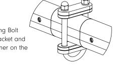
Reinsert the Locking Bolt and tighten the bolts firmly – until you notice the rubber beginning to squeeze – to secure the Rail Bracket.
