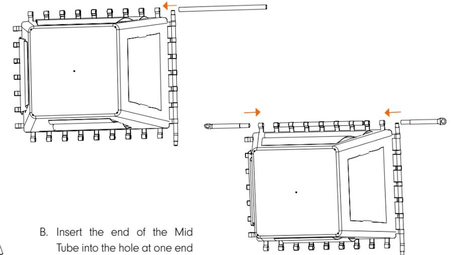
B. Insert the end of the Mid Tube into the hole at one end of the Base Joiner.
