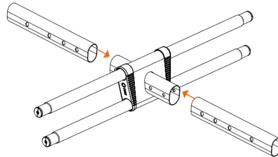
B. Insert an End Joiner into the centre of the other H Joiner (or both ends, if you will later attach Swing Set frames to both ends of your Cubby House). Lock them together with Frame Bolts.
